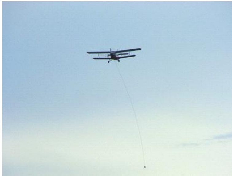
Figure 1. EM-4H installed on the An-3
