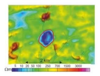
Figure 3. Resistivity map for 3163 Hz frequency channel for large (~ 1000 m) non-magnetic diamond kimberlite body (red circle) in Lunda Norte province (Angola).
