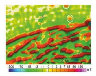
Figure 4. Local part of anomaly magnetic field map for large (~ 1000 m) non-magnetic diamond kimberlite body (red circle) in Lunda Norte province (Angola).
