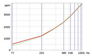
Figure 7. Measured quadrature response (red) for 77 Hz is 150 ppm greater then modeled one over the same medium without deep conductor (green)
