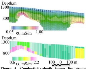
Figure 5. Conductivity-depth image for ground survey data (upper image) and 2 layer inversion results (bottom image) for EQUATOR data over Ergoju deposits (deposits fit perfectly with conductive areas).
