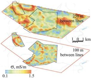
Figure 4. Conductivity map after EQUATOR survey (upper image) and ground survey data (bottom image).
