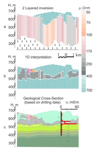
Figure 4. EM4H interpretation: a) 2 layered inversion; b) 1D interpretation; c) geological cross-section with conductivity log results (red chart)
