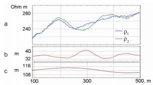
Figure 1. Receiver positioning results: a) apparent resistivity calculated using actual bird position ( $\rho_1$ ) and using average offset ( $\rho_2$ ); b) vertical bird offset – affects  $\rho_2$  deviation about 10%; c) aircraft altitude – no influence on apparent resistivity
