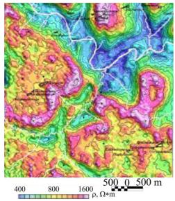
Figure 5. Apparent resistivity map at 520 Hz.
