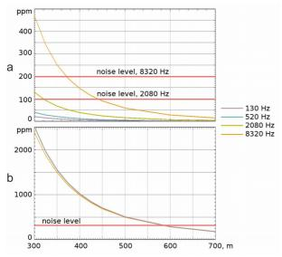
Figure 2. EM4H sensitivity over salt lake: response modelling data as a function of altitude (water: 4 m, 12.5 S/m; basement: 10 mS/m). a) Quadrature response – altitude limit for noise level is 380 m. b) In-phase response – altitude limit for noise level is 600 m
