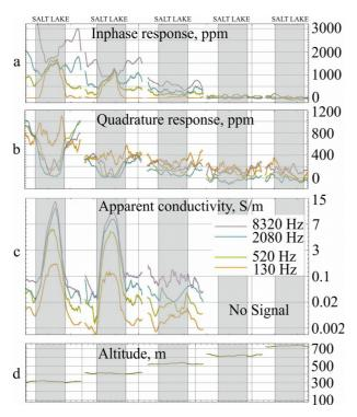
Figure 3. EM4H sensitivity over salt lake (marked in grey): flight data as a function of altitude. a) In phase response; b) Quadrature response; c) Apparent conductivity: lake is not detected at 500 m, ground is not detected at 600 m and higher; d) Altitude.
