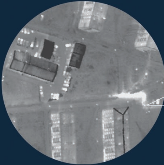
Monitoring of heat supply network. Infrared image and the result of 'anomaly check'. Infrared survey in Riga.
