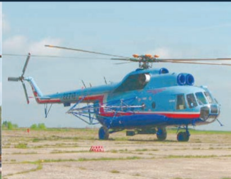
EM4H installed on Mi8 (Aerogeophysica Inc.)
